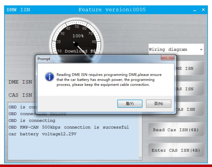
Make sure the battery has enough power and not disconnected
