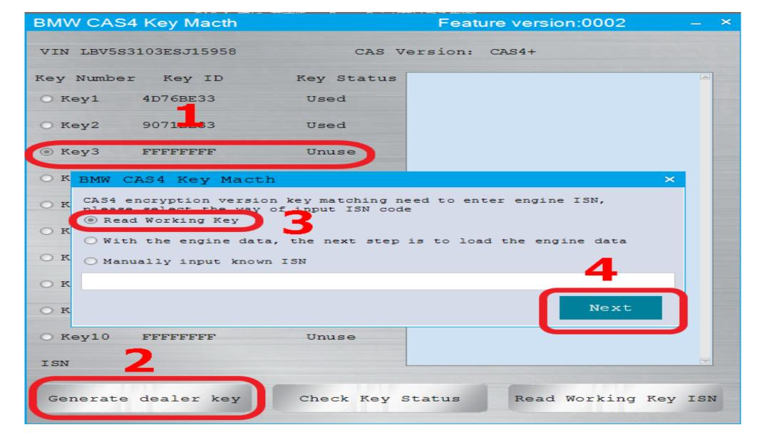
Select the key position that needs to be configured, click to generate the dealer key, and click on the engine data to determine the next step
