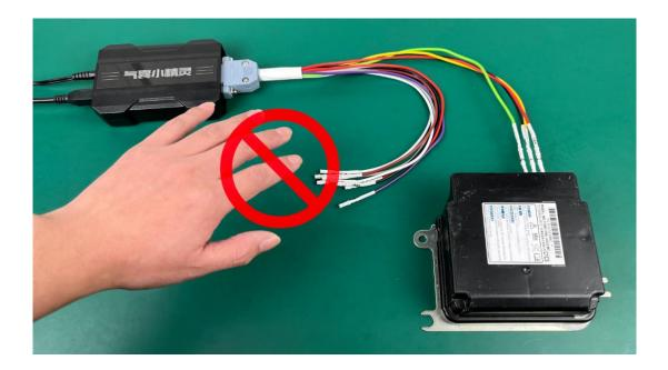
When some airbag ecu are being repaired, the CG70 will read the original EEPROM data, which must be saved for subsequent maintenance.
