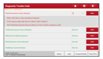
The tested system with fault code appears in red and the system with OK displays in black (normally).
