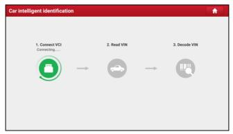
Note: If the VCI is not paired up with the tablet before doing this step, a prompt message box will appear on the screen. Check all the possible reasons of Bluetooth connection failure carefully, and then tap **OK** to the following screen.
