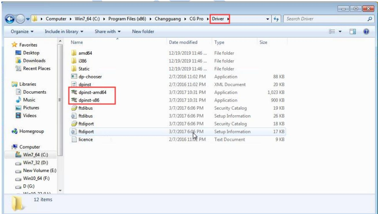
For the WINXP system, look for the installed driver in the Driver\_xp folder. The 64-bit system is equipped with DPInstx64.exe; the 32-bit system is equipped with DPInstx86.exe. As shown below:
