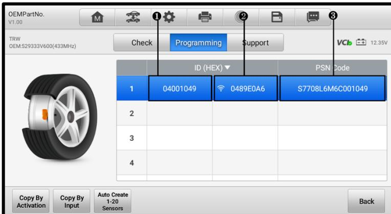
**Figure 6-44 Programming Screen via OEM Part NO.**
