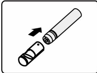
2. Slip the end of the accessory over the imager head and then fix the accessory.
