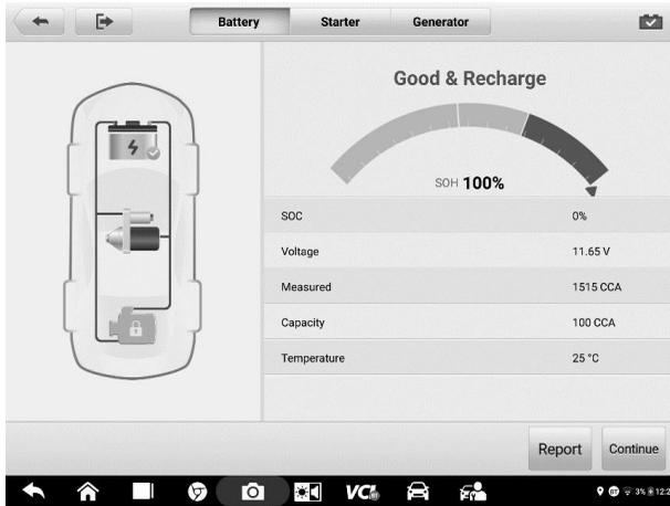
**Figure 10-6 Battery Test Results Screen**
