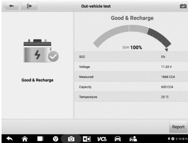
Figure 10-10 Out-vehicle Test Results Screen
