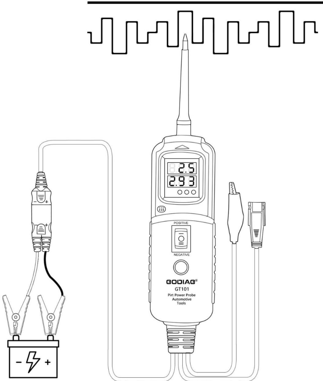
*Note: The insulated wire needs to be pierced into and connected to the copper wire by the probe before it can be detected.*
