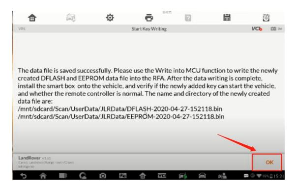
Then go back to the menu Read/write chip Data to write the new created Dflash file and EEPROM file back to the MCU.
