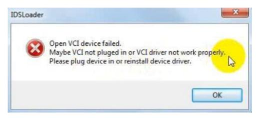
• when you put FVDI J2534 equipment to connect the computer and open the software, it will pop below error message, it means you do not connected vehicle ECU module and the ECU voltage can not less than 8 volts. After using the OBD interface of FVDI J2534 to connect the ECU, and the software can be opened normally and put into use.
