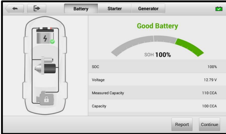
Figure 12-7 Battery Test Results Screen
