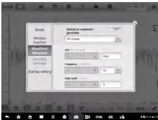
Figure 9-25 Waveform Generator Screen
