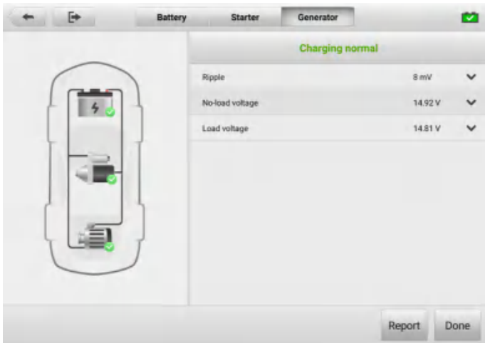
Figure 20-8 Generator Test Results Screen
