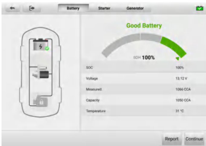
Figure 20-6 Battery Test Results Screen
