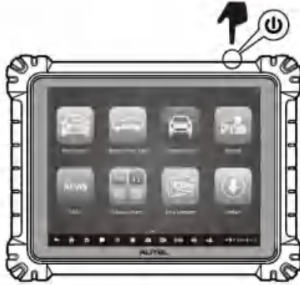
Figure 5-3 Power up the Tablet
