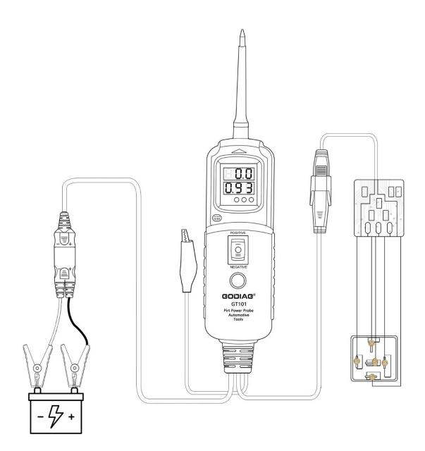
B. For relays with only normally open function, the red power light on the relay adapter flashes; for the normally open, the green light flashes; for the normally closed, the blue light goes out. The current shows the normal current value.
