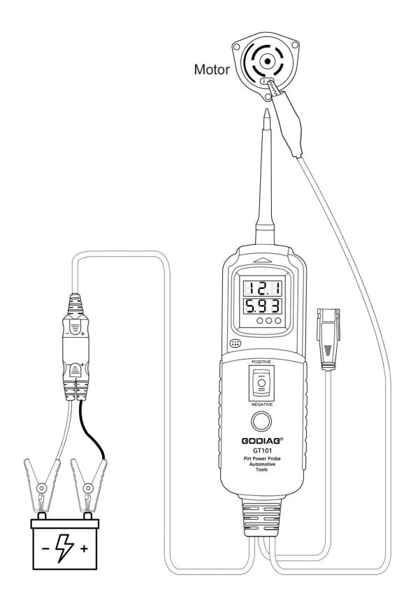
Negative circuit module and component circuit activation test. Find the GND connection of the vehicle module according to the circuit schematic diagram. After the probe touches GND, the red LED light should light. The buzzer makes a rapid sound, the voltmeter displays the current voltage, and the function switch is pressed backward to output the
