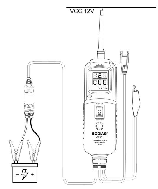
C. GND/battery negative or ground detection: When the probe detects that the current circuit is battery negative or ground GND, the device will emit a low-frequency sound, the corresponding GND indicator will flash; and the voltmeter will display 0V.
