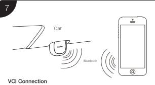
For Android devices, tap Me > VCI Connection or the VCI button near the top right of the Home screen. For iOS devices, tap Setting > Bluetooth on your iOS device to open the Bluetooth function. Then tap the Bluetooth name of the MaxiAP AP200 tool to pair it with the device. The Bluetooth name starts with AP, followed by the serial number of the tool.
