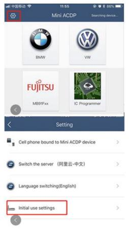
3. Following the directions: press and hold the "SET" button on the ACDP device for about 7s till the device's buzzer sounds, then release the "SET" button. Then click "Next"
