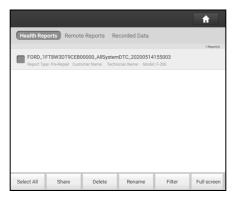
All diagnostic reports are sorted by Date and Make. Tap the desired type to re-arrange and filter it.
