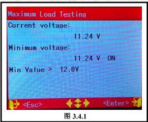
Follow the prompts, first open all the electrical equipment, and then start the engine after waiting for about 15 seconds waiting for the stable operation of the engine press <Enter> to start testing, intrusion detection interface (Figure 3.4.1).
