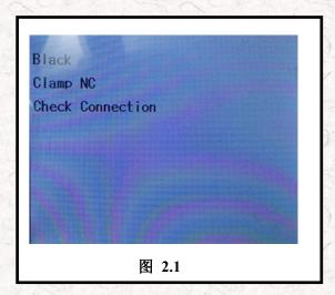
2. wiring to normal after device initialization is successful, the display will automatically boot interface (as shown below), press any key to continue.
