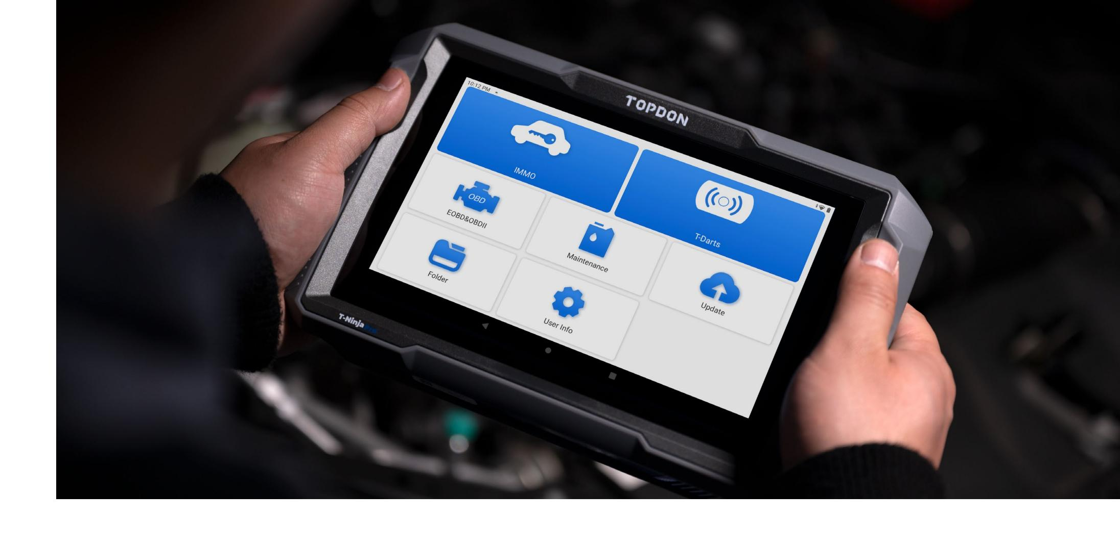
upgrade to the T-Ninja1000, the T-Ninja Pro boasts a variety of functions, including Number of Keys, PIN Reading, Key Learning, Remote Control Learning, Delete Keys, and All Keys Lost. Supporting full OBD2 functions and 8 maintenance services, this key programmer also works as an OBD2 scanner and helps technicians perform essential diagnoses on cars.
